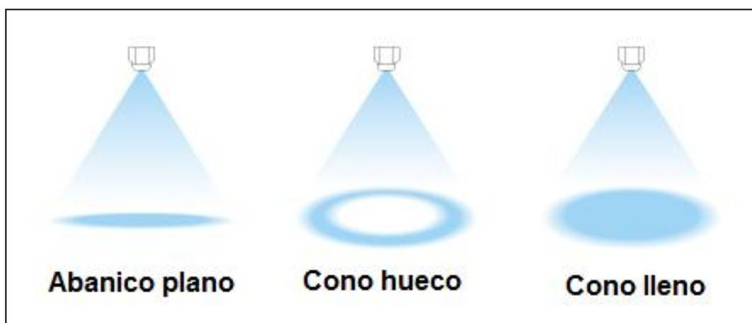
Figura 1: Patrones de distribución. Adaptado de [www.ikeuchiusa.com/technical\\_information.html](http://www.ikeuchiusa.com/technical_information.html)
